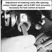
figure from the Mohegan Sun Top Fuel Dragster is a Pete Jackson valve. It is uniquely engineered for an instantaneous surge of fuel at the launch. In the
