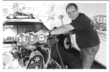
Larry Higginbottham's using his favorite tool on his potent Top Sportsman '96 Corvette with a 526 cubic inch, blown alcohol Big Block; running a special 3 speed automatic transmission based on the turbo 400. Higginbotham qualified at Norwalk with a 6.43 at 209 MPH; what a run for a full-bodied drag racer. Larry is making a secret adjustment, caught with our spy-cam. Don't tell him.
