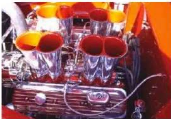
Sharp MFI setup on a street rod show car. Fuel injection is great on an engine built for the show market where outside appearance stimulates emotion.
