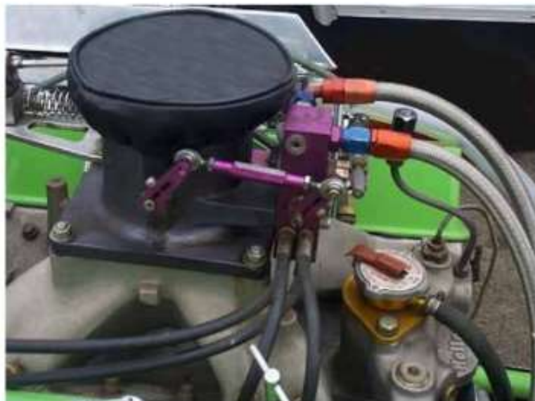
Simple throttle body MFI setup from Rons Fuel Injection – popular in custom engine builds, especially for drag racing.
