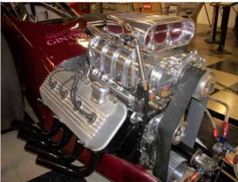
Vintage blown early Hemi with Roots supercharger and Enderle fuel injection is common in Nostalgia drag racing.
