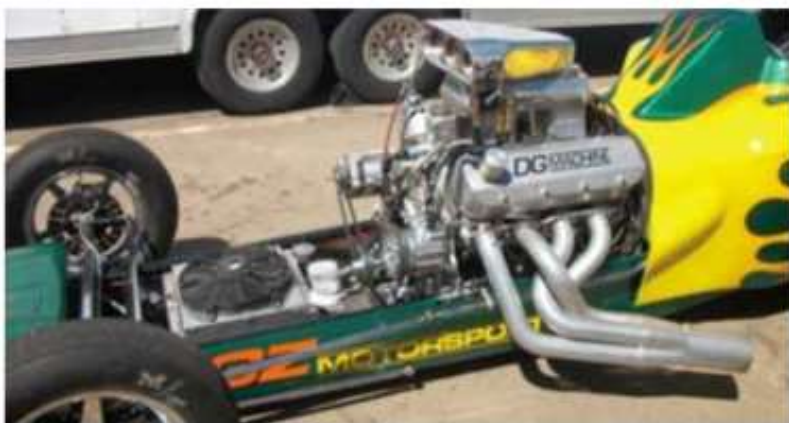
A hat type of fuel injection on a tunnel ram manifold makes an impressive looking combination. Grass roots racers are often dependent on an experienced engine builder to sort out jetting for this combination.
